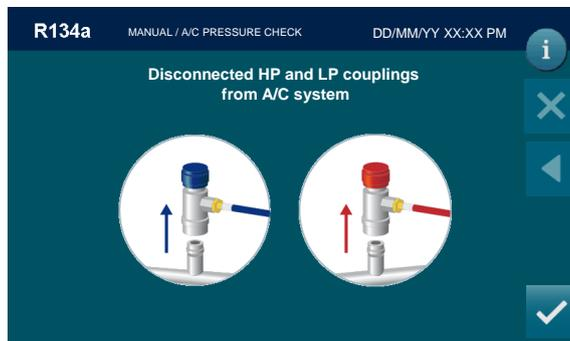
Disconnect coupling from A/C system, press
