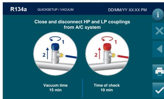
Close and disconnect HP and LP coupling from A/C system, then press
