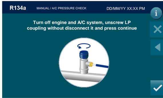
Turn off engine and A/C system, unscrew LP coupling without disconnect it, then press
