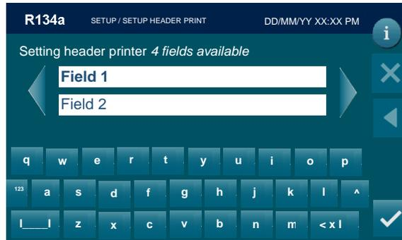
Use the keypad to modify the 4 lines, then press
