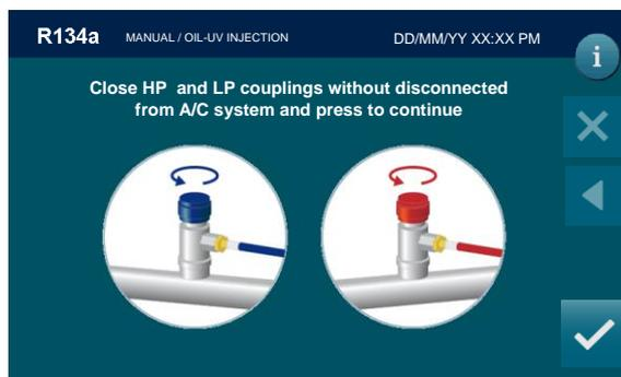
Unscrew HP and LP coupling without disconnect from A/C system end press
