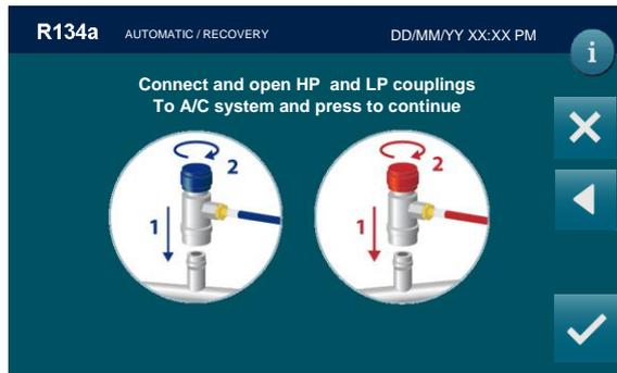
Connect and open HP and LP couplings (or those chosen in the previous point) to A/C system and press
