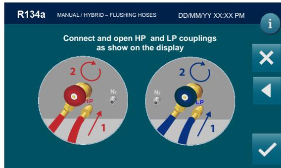
Connect the HP and LP couplers to the respective fitting on the machine, the press
