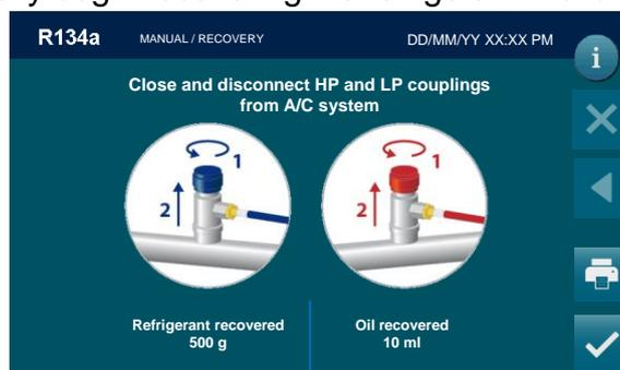
Unscrew and disconnect HP and LP coupling from A/C system end press
