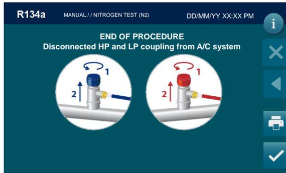
Unscrew and disconnect HP and LP coupling from A/C system end press
