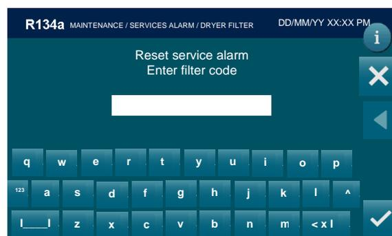
7) Type the filter code and press
