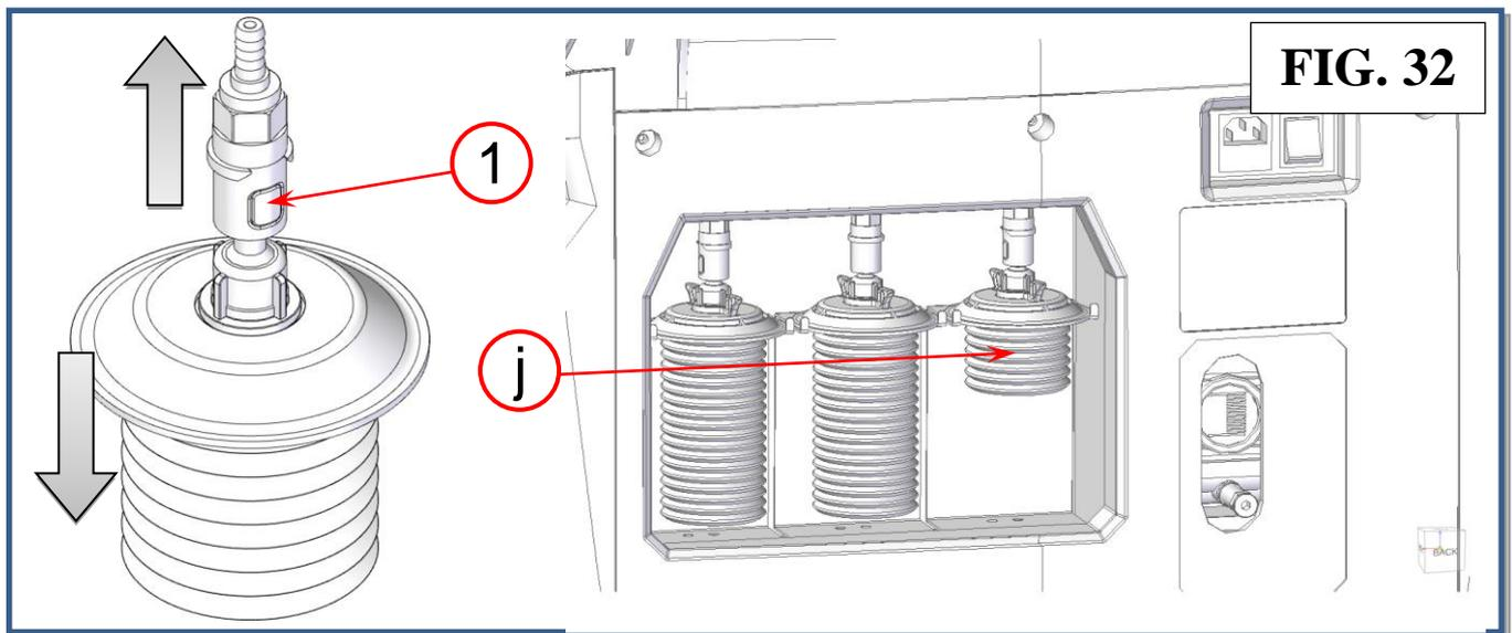
1. Insert the male insert of the new DYE cartridge into the quick connection and replace the cartridge in its housing.
