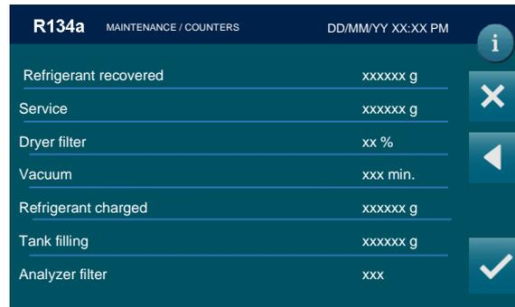
The screenshot shows a dark teal interface for the R134a MAINTENANCE / COUNTERS screen. At the top, it displays 'R134a MAINTENANCE / COUNTERS' and a date/time 'DD/MM/YY XX:XX PM'. Below this is a list of seven counter items, each with a value and a unit. On the right side of the list, there are four navigation icons: an information icon (i), a close icon (X), a left arrow, and a checkmark icon.
