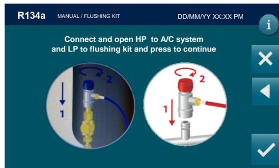
Connect and open HP to A/C system and LP to flushing kit and press
