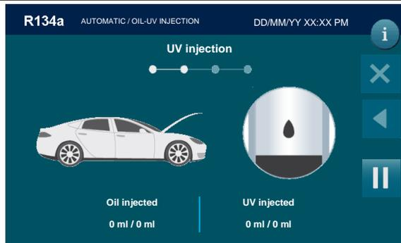
When completed, the system will go on to charging with the preset quantity of refrigerant.
