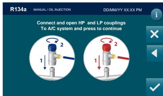
Connect and open the coupling (HP, LP, or HP/LP, depend of the previous choice) connected
