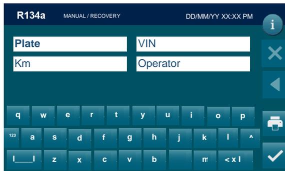
Type the plate of the car, VIN, Km, Operator and press
