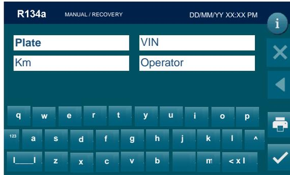
Type the plate of the car, VIN, Km, Operator and press
