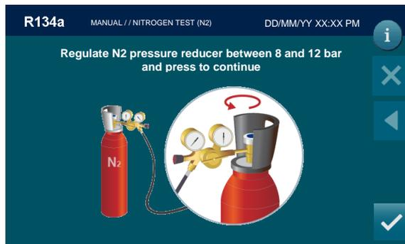
Regulate N2 pressure reducer between 8 and 12 bar and press  :
