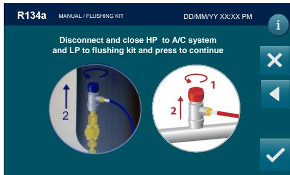
Disconnect all the couplings and press
