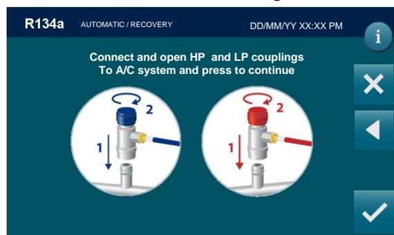
Connect and open the coupling to the A/C system, then press
