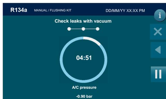
The machine check leaks with vacuum
