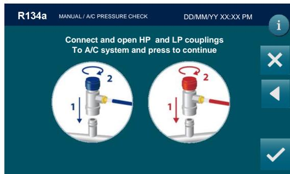
Connect and open the coupling connected to the A/C system, then press
