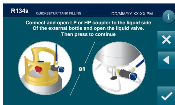
Connect and open LP or HP coupler to the liquid side of the external bottle and open the liquid valve. Then press
