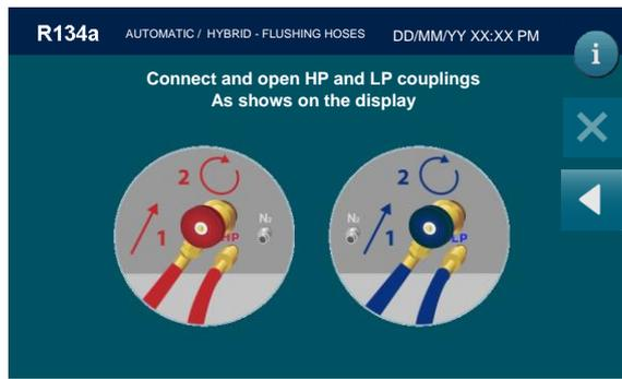
If HYBRID VEHICLE is selected the machine will perform FLUSHING HOSES
