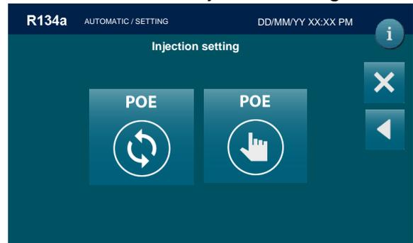
Select PAG/POE oil symbol AUTOMATIC injection
