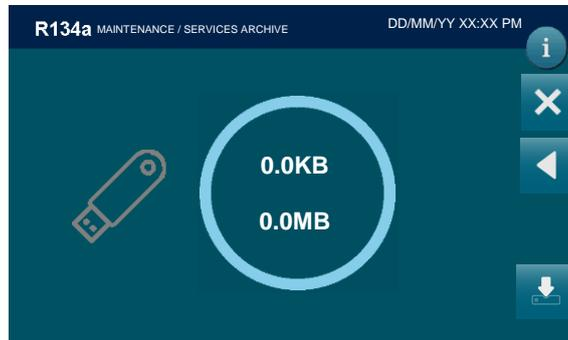
Insert the storage device in the USB port the available space of the usb pen will be displayed
