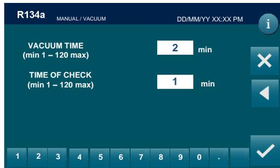
use the KEYPAD to insert the new value of the VACUUM TIME, press
