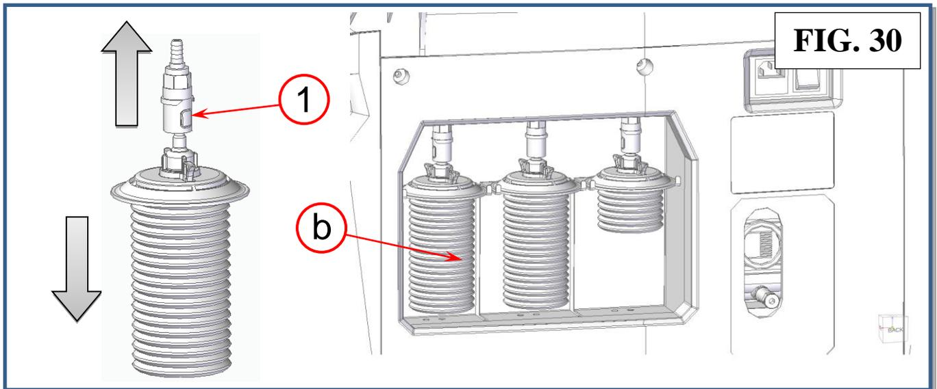
1. Insert the male insert of the new oil cartridge into the quick connection and replace the cartridge in its housing.
