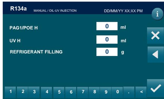
Use the keys 0 to 9 to type the volume of UV to be injected, can never be more than 10 ml.
