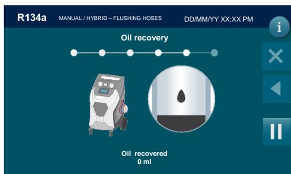
The machine automatically displaying the used oil extracted
