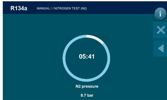
If leaks are detected, the machine will give an alarm signal, discharge the nitrogen from the system, and display a SYSTEM LEAKS alarm warning. If the test detects no leaks, the machine will discharge the nitrogen:
