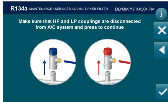
Make sure that HP and LP coupling are disconnected from A/C system or else and press
