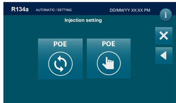
Select PAG/POE oil symbol AUTOMATIC injection
