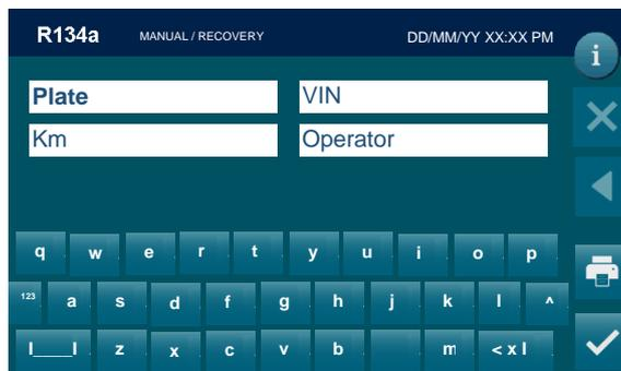
Type the plate of the car, VIN, Km, Operator and press
