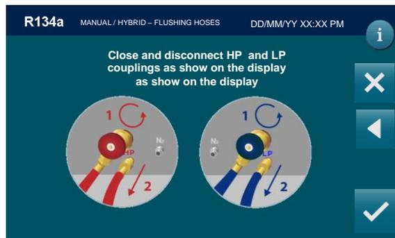
Close and disconnect coupling, then press
