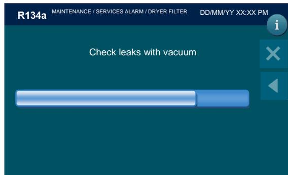
automatically the machine proceeds to the pressure control
