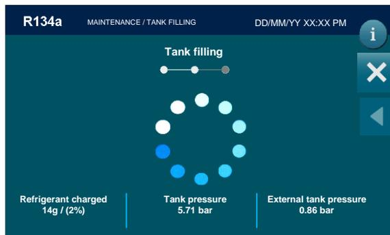
the machine will now fill the machine tank with the preset quantity ~ 500g. When the quantity minus 500 grams is reached, the machine will stop and display:
