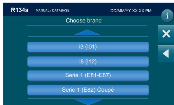
Select the model of vehicle you are servicing. (If you wish to install DATABASE contact the machine dealer.), all the information about this model is displayed:
