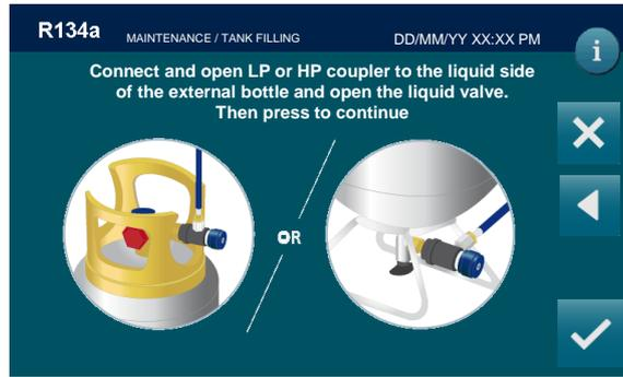
Procure a bottle of appropriate refrigerant (R134a or R1234yf depending on machine model), connect and open LP or HP coupler to the liquid side of the external bottle and open the liquid valve, then press . The BOTTLE FILLING will start
