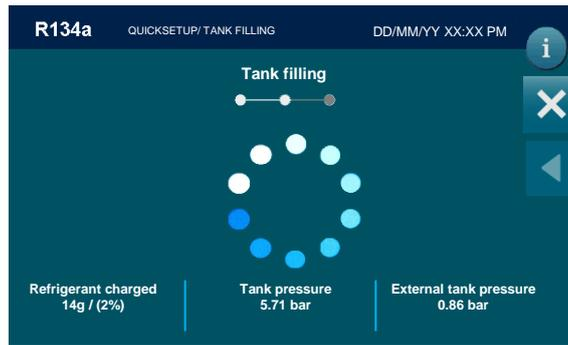
The machine will proceed automatically, displaying the quantity of refrigerant charged in the tank. When filling is completed, the following screen is displayed:
