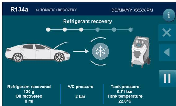
During the recovery phase, the machine displays the quantity of refrigerant recovered, in grams. Upon completion of recovery, the machine will stop and discharge, while automatically displaying the used oil extracted from the A/C system during the recovery phase.
