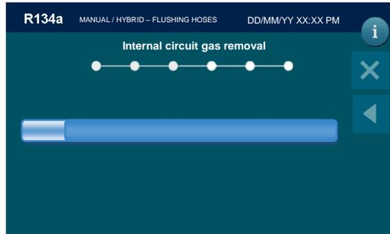
Flushing hoses lasts few minutes, then the machine will sound and alarm and the following screen will be displayed:
