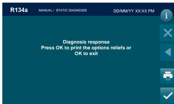
Press OK to print the diagnosis report: should the diagnosis results not be positive, the printout will list from one to three possible system problems. When checking, always start with the first DIAGNOSIS shown and check each in the order given, applying the REMEDIES listed for each DIAGNOSIS.
