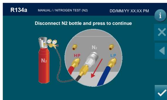
Disconnect coupling, then press
