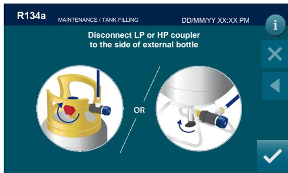
Close the liquid valve of the external bottle and press , the machine will recover the residual refrigerant from the hoses, then will display the following screen:
