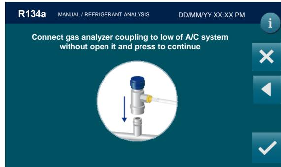
Connect gas analyzer coupling to low of A/C system
