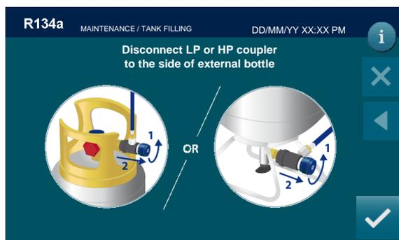
Close and disconnect LP coupling from external bottle and press .Bottle filling procedure successfully completed. Switch the machine off.
