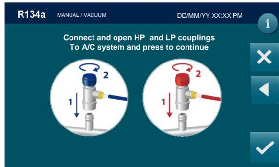
Connect and open the coupling connected to the A/C system, then press
