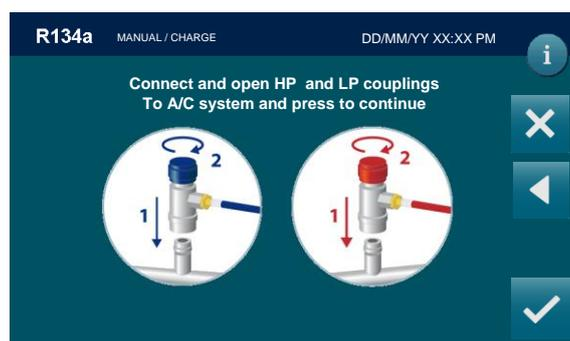
Connect and open the coupling (HP, LP, or HP/LP, depend of the previous choice) connected to the A/C system, then press
