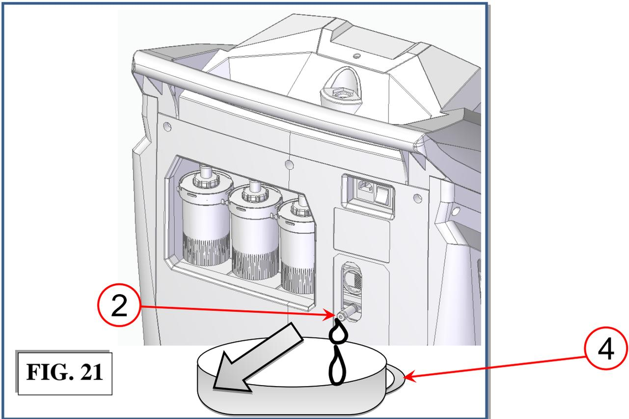
Allow all the oil to run out into a disposal container (ref 4 Fig.21) (with height < 10 cm).
