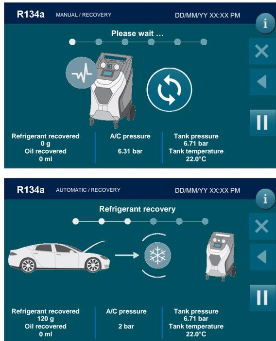
During the recovery phase, the machine displays the quantity of refrigerant recovered, in grams. Upon completion of recovery, the machine will stop and discharge, while automatically displaying the used oil extracted from the A/C system during the recovery phase. The oil discharge operation lasts 4 minutes.
