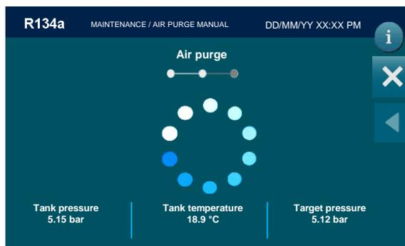
Automatically the machine will start to discharge the air up to the target pressure.
