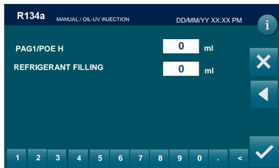
Use the keys 0 to 9 to type the volume of oil to be injected.
