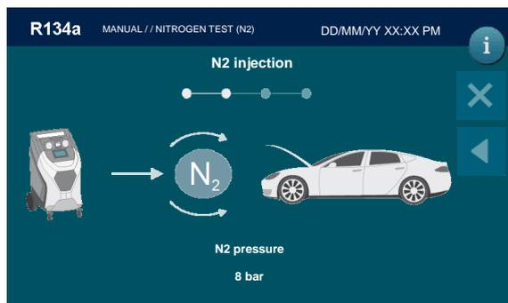
The nitrogen will be injected into the A/C system, the test will start as soon as the pressure is stable:
