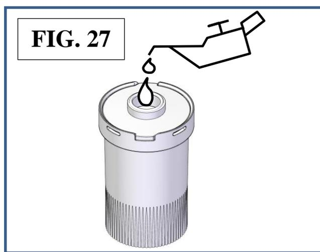
**NOTE:** in order to reduce humidity and air contamination of new oil, the collapsible container has to be filled almost to the brim.
