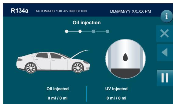
the quantity of UV set by the operator will be automatically reintegrated.
