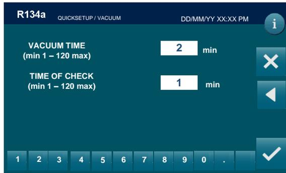
Use the KEYPAD to insert the value of the VACUUM TIME, press
