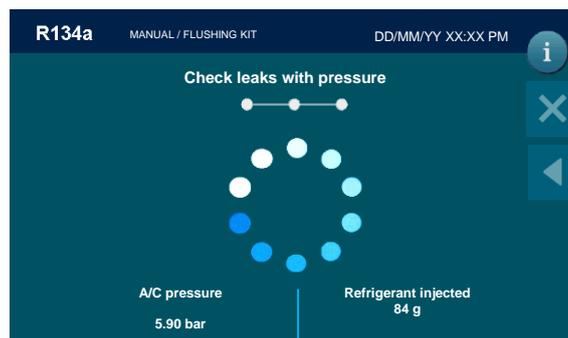
The machine check leaks with pressure
