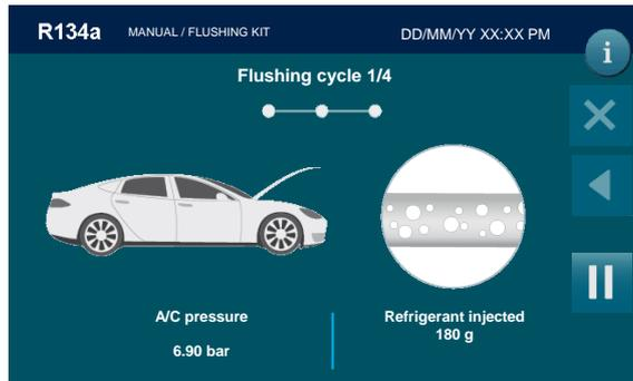
The machine will proceed automatically to 4 flushing cycle
