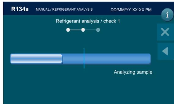
The machine performs an internal calibration before performing the measurement.
