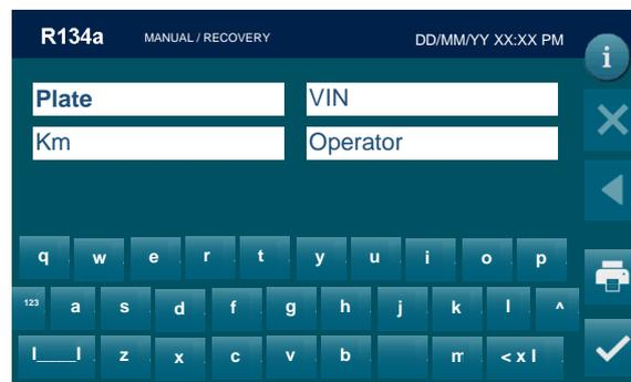
Type the plate of the car, VIN, Km, Operator and press
