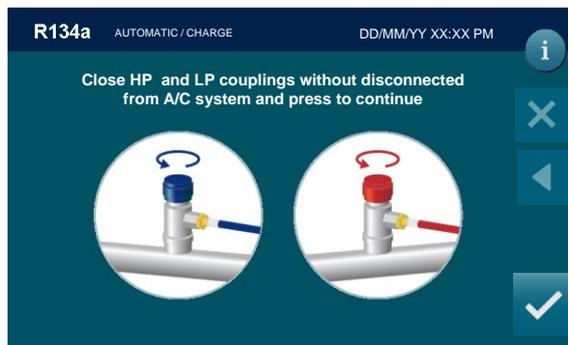
Unscrew HP and LP coupling without disconnect from A/C system end press
