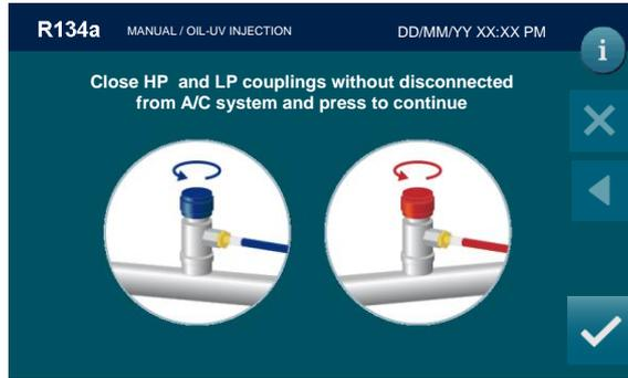
Unscrew HP and LP coupling without disconnect from A/C system end press
