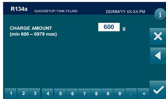
Use the touchscreen keys 0 to 9 to type the quantity (in grams) of refrigerant to be charged into the tank, then press
