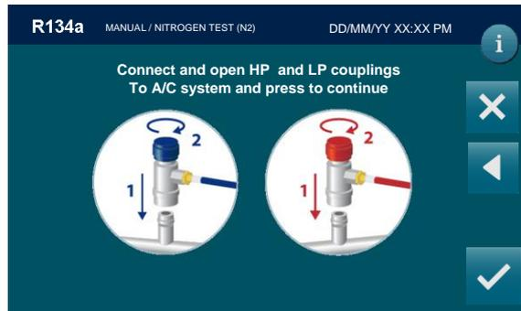
Connect and open HP and LP coupling to A/C system, then press OK to continue; the following screen will be displayed:
