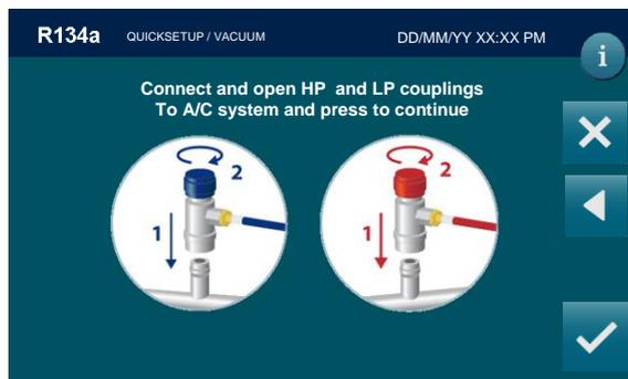
Connect and open the coupling connected to the A/C system, then press
