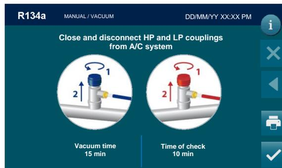
Close and disconnect HP and LP coupling from A/C system, then press
