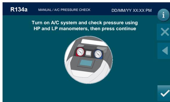
Turn on A/C system and check pressure using HP and LP manometers, then press
