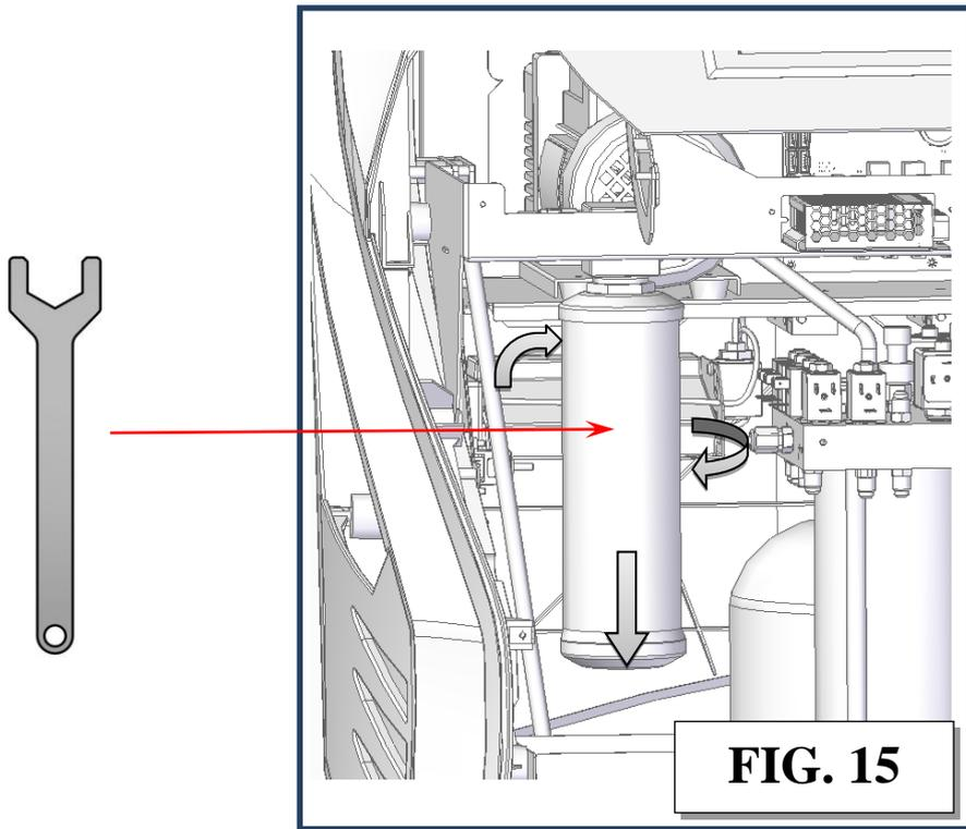
9) Take the new filter, wet with clean POE oil both o-rings, and verify that they are correctly placed into their seats
