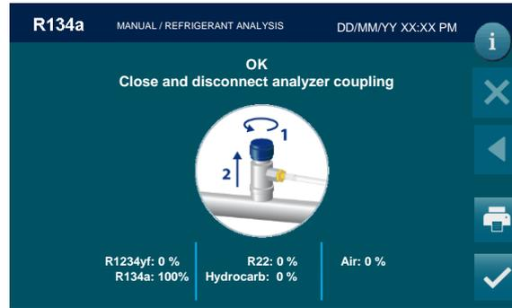
Close and disconnect analyzer coupling
